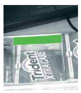
(B) The pixel counter detects if one layer is missing by means of the visible area at the inside of the cardboard box
