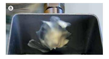
(A) The LMT sensor monitors the level of mayonnaise using the high-frequency capacitance spectrum profiling technology. (B) Despite deposits on the sensor the empty tank is detected reliably.
