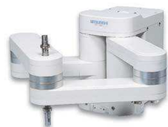
SCARA robots are ideal for applications where space is limited.
