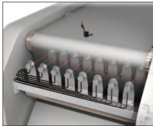
8 fiberoptic sensors used
