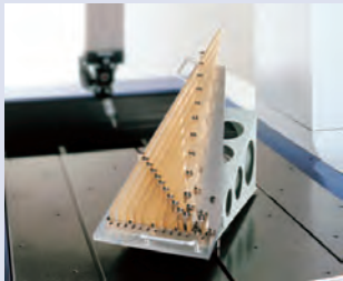
CMM calibration using a virtually zero thermal expansion glass gauge
