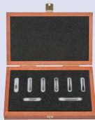
CMM calibration using a virtually zero thermal expansion glass gauge
