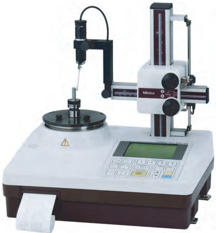
RA-10 with optional X-axis stop and Z-axis scale unit
