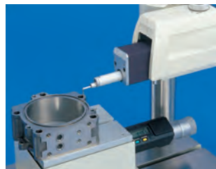
Deep groove measurement
