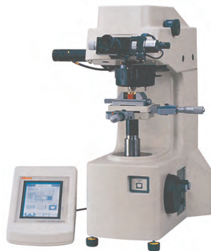
HM-112 Digital display of measurement results and a statistical calculation function
