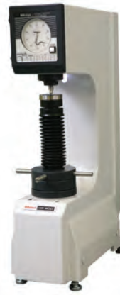
HR-210MR Rockwell hardness testing machine Manual weight changing (with total test force selected) and handling of preload force. Motor drive controls loading sequence.
