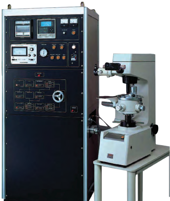
AVK-HF / 810-155 Vickers hardness testing at high temperatures.
