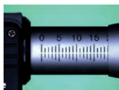
Field of view with QI-A 0.2X magnification
