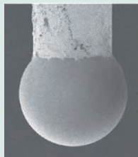
UMAP 110 \phi 100 \mu\text{m} L = 10 mm
