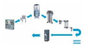
Complying with the Rule Requirements of the classification societies, our Custom Design Department has designed for you the N<sub>2</sub> capacity you need, built on a single skid. It comes complete with compressor, after-coolers, filters, air receivers, dryers and N<sub>2</sub> units to match your available footprint. An N<sub>2</sub> receiver can be provided as an option.
